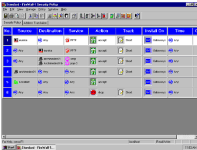
Figure 13.1: Firewall-1's rule-based interface
