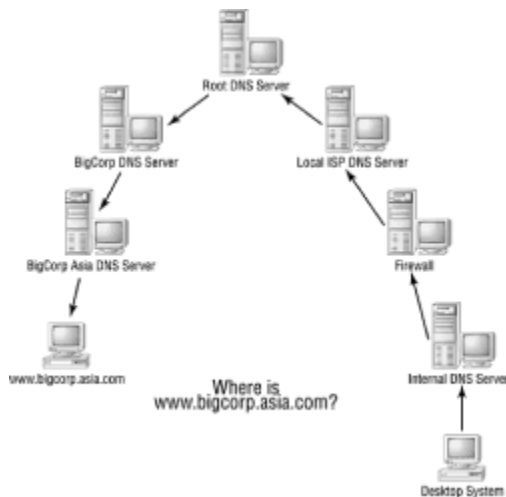
Figure 4.1: The DNS system distributes control of Internet domain names.
